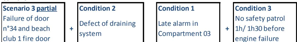
Combination 1: beach club 1 is considered as the first compartment to be flooded. The height of water observed (1 m), could seem to be quite high considering the relatively little hydrostatic pressure difference between the inside and the outside of the vessel. Thus all the water flooding should not stay in the beach club 1, unless the stern sinkage becomes very important, which was not the case, as it seems when the investigation had been done.
