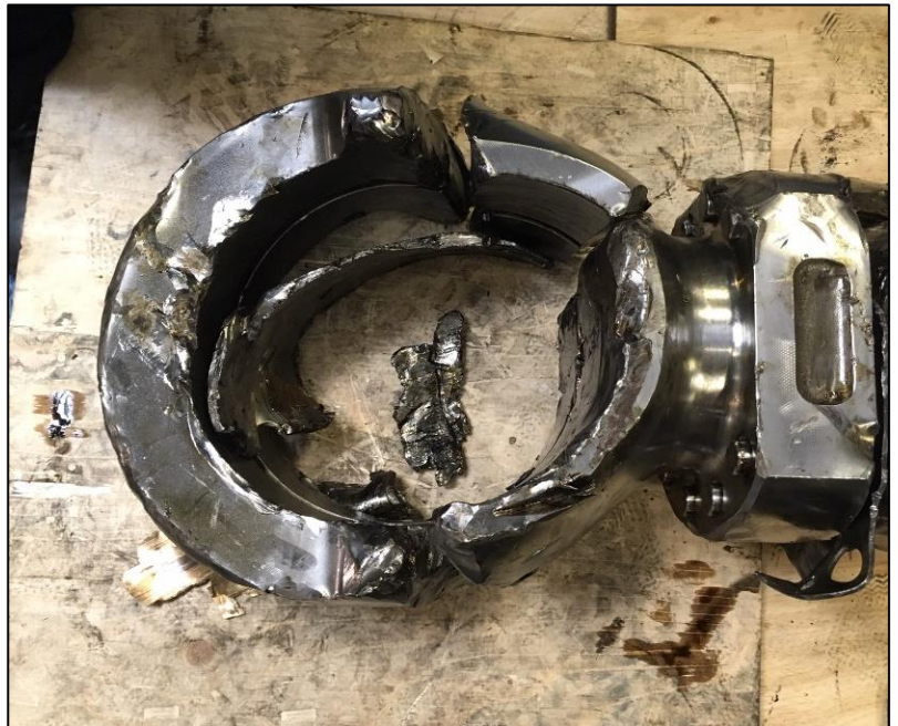
Connecting rod small-end of the A5 cylinder after the accident
