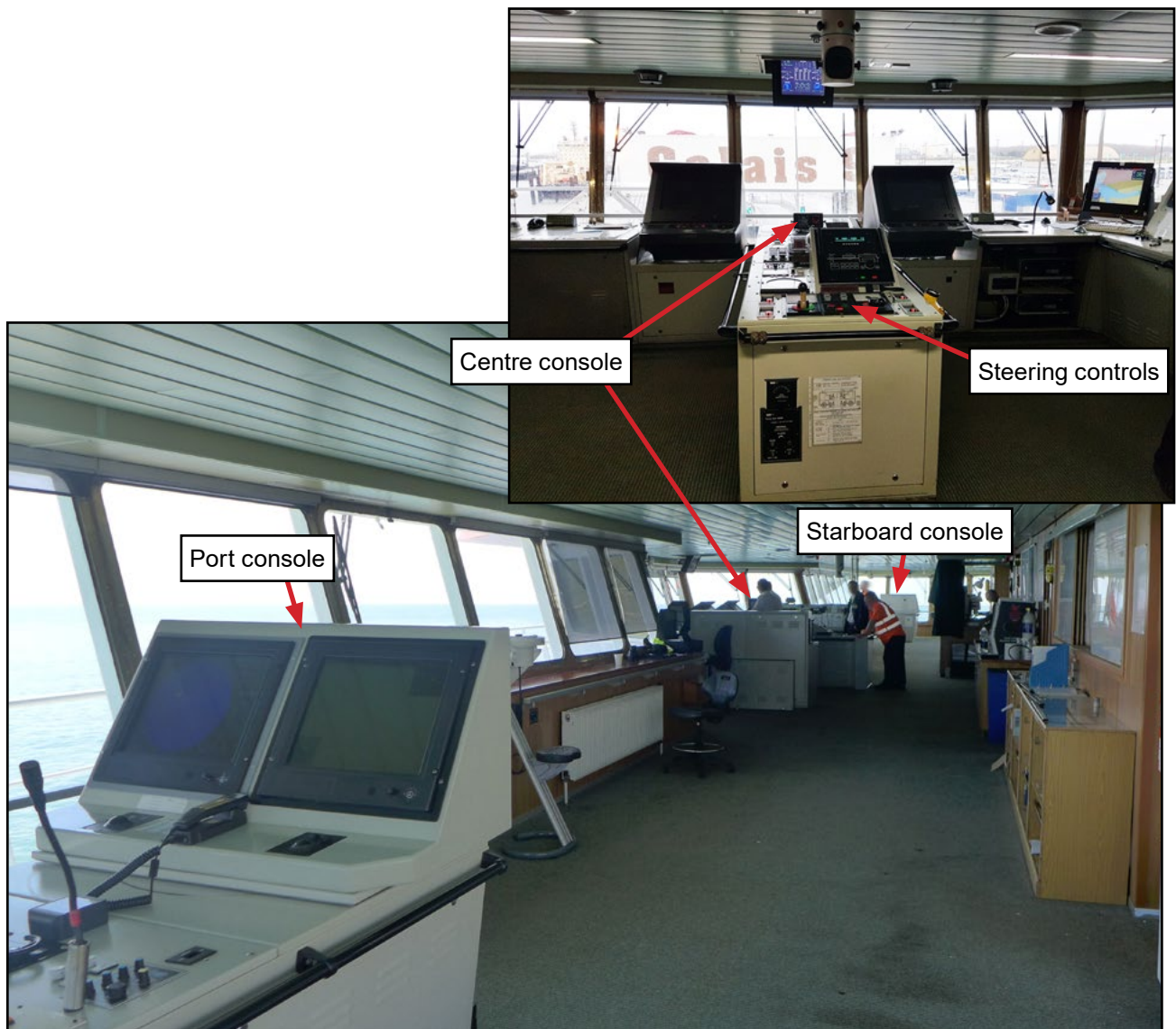
Figure 9: Fully enclosed bridge arrangement
