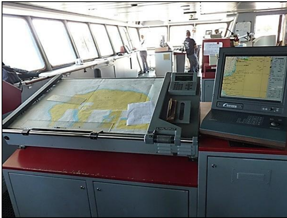
The wheelhouse console located on starboard with the plotter on the left and the ECS on the right.
