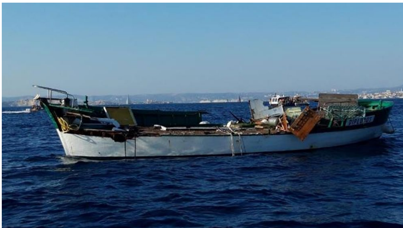
Figure 19 : View of Diplodus on her port side after being hit by Sky Fall. Source: amateur photographer, to be compared with the photo of the vessel with her superstructure before the accident at the beginning of this report (Figure 16).
