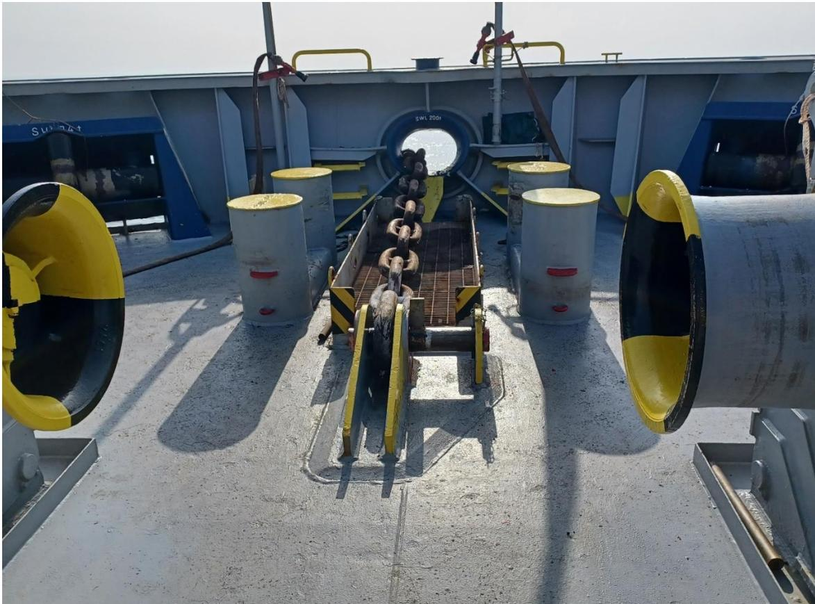
Figure 2 – Towing chain connected to the "Smit Bracket"
