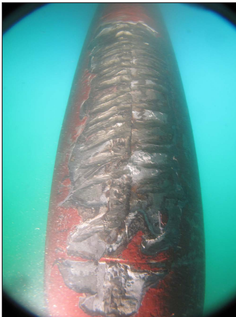
Figure 3a: Damage to Barfleur's port rudder
