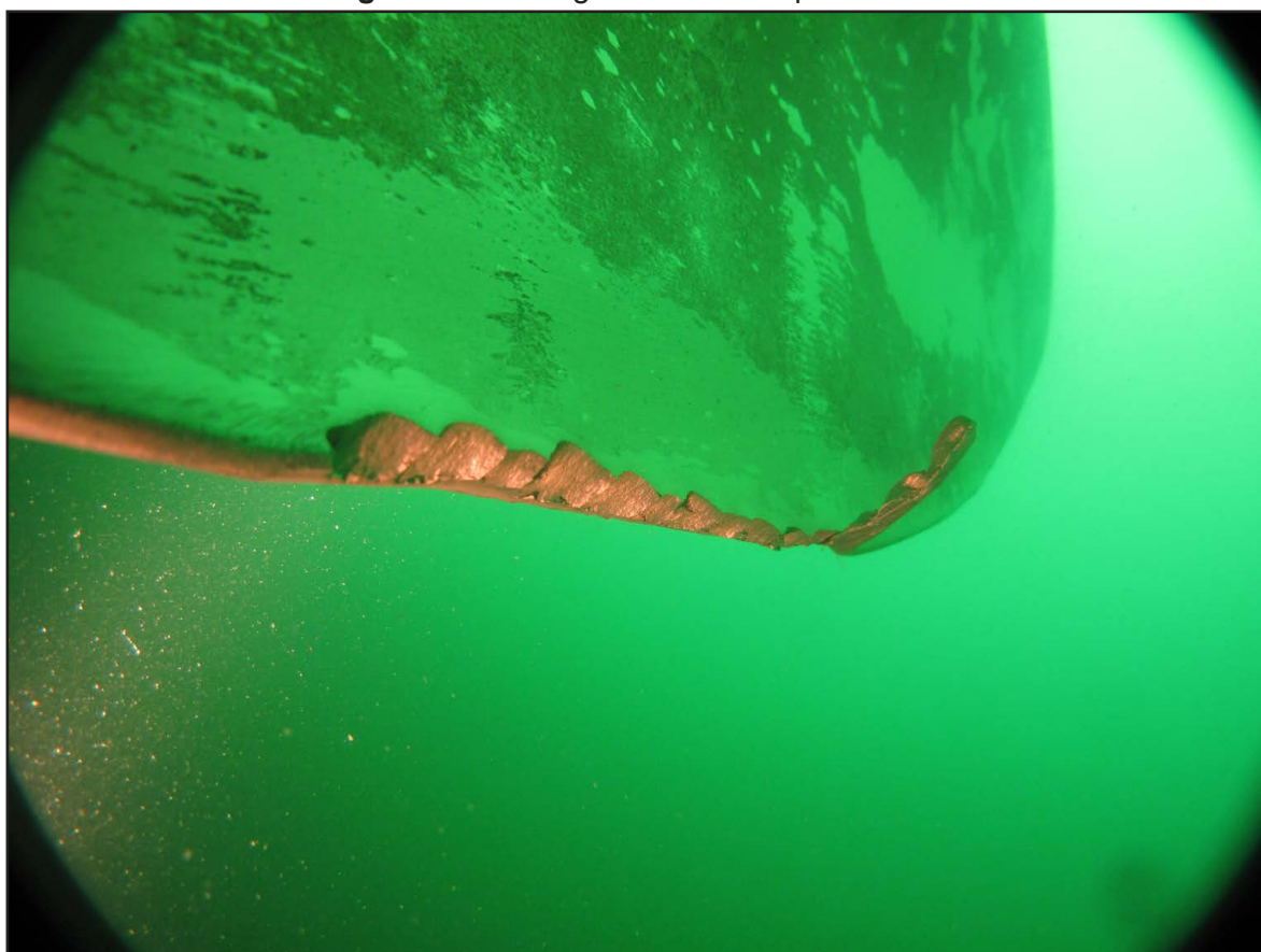
Figure 3b: Damage to Barfleur's starboard propeller
