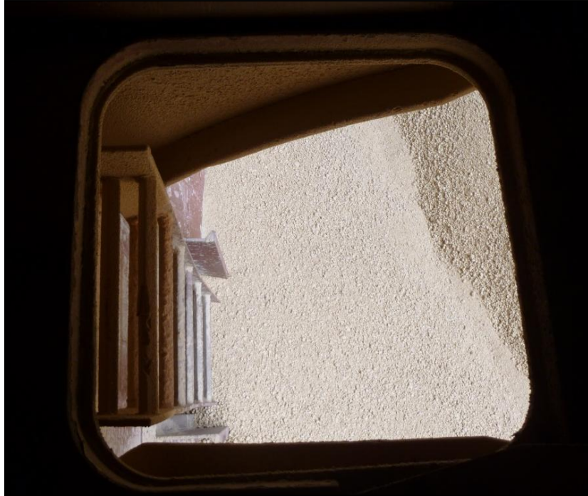
Figure 8: Lower vertical ladder giving access to the cargo space
