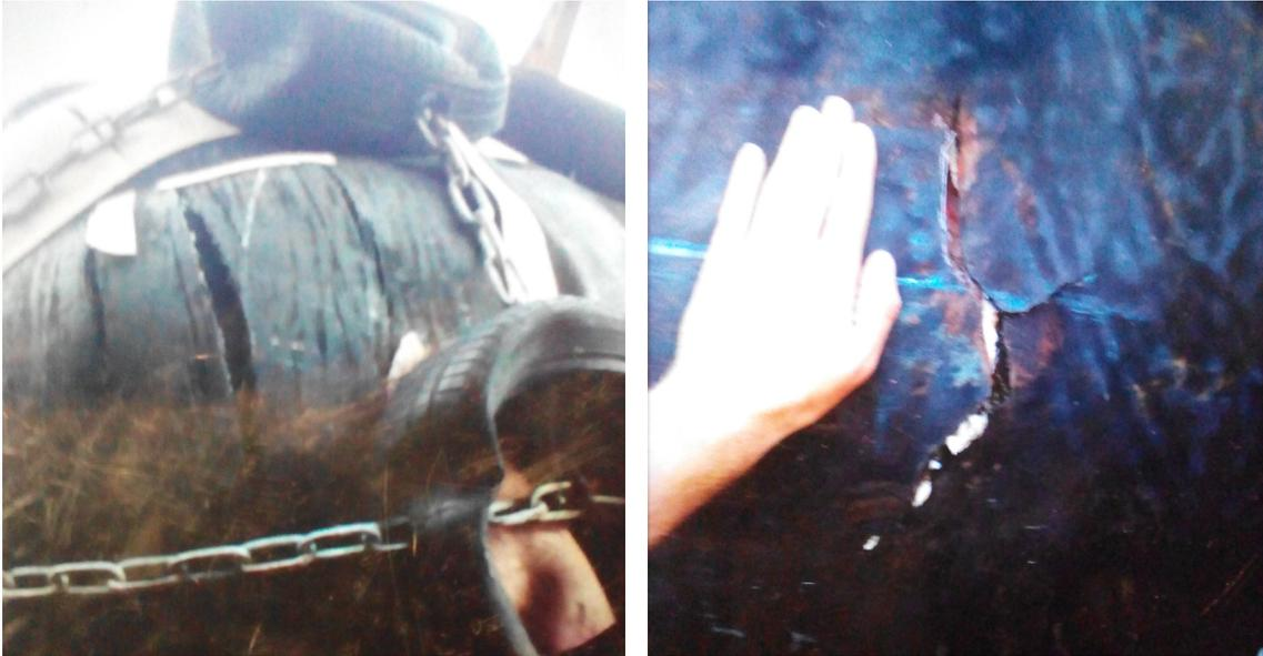
Figure 14: Photos showing details of wear and damage to the fenders upon delivery.
