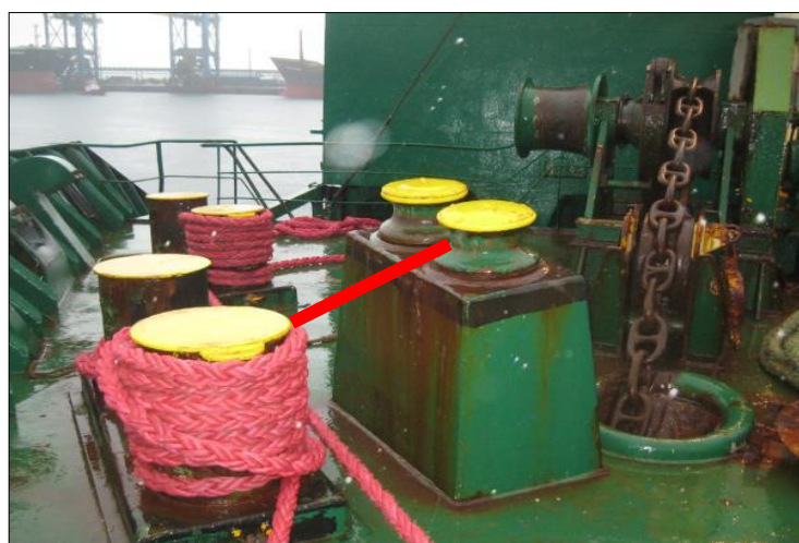
Figure 7: Different heights of mooring equipment on the forecastle deck (red line indicates the resulting angle of the mooring rope)
