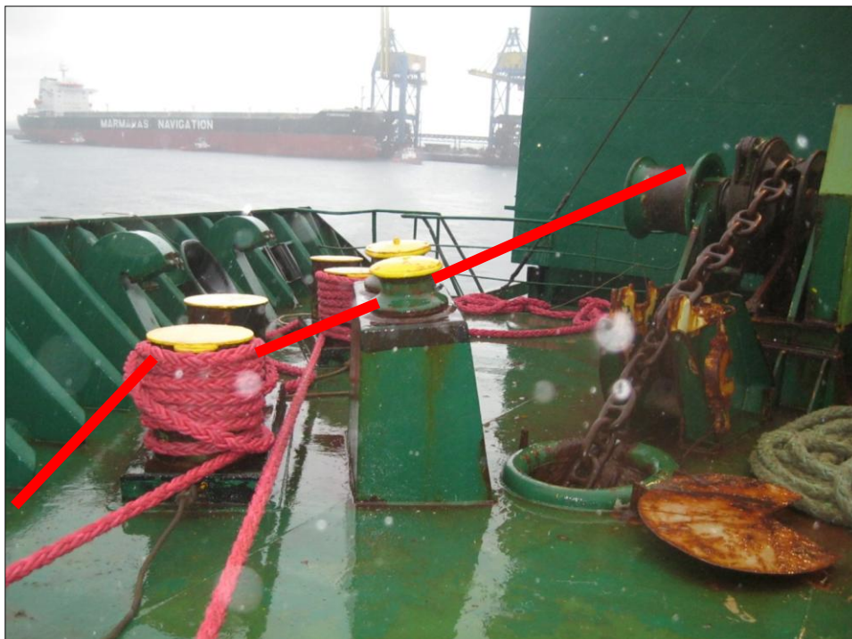
Figure 5: The head line arrangement at the bitts and the pedestal fairleads
