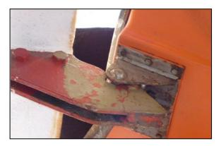
Figure 4: The hook, which keeps the lifeboat in position
