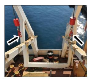
Figure 3: Port and starboard falls and hooks
