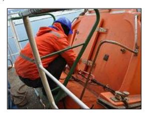
Figure 7: One of the crew member removing the aft lashings in order to gain access into the lifeboat
