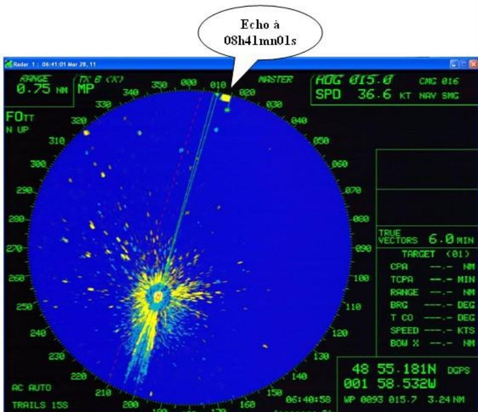
From **8:41:01 am** to **8:42:20 am**, (Course made good  $013.8^\circ$  - Speed made good 36.7 knots) the potter blip was closing quickly *CONDOR VITESSE*. At first it had moved away to the right from the HSC track then it got closer again.
