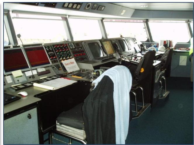
The panoramic wheelhouse takes up the full width of the bridge deck. The control position is ergonomic. Two wings extend the bridge and have opening lateral windows.
